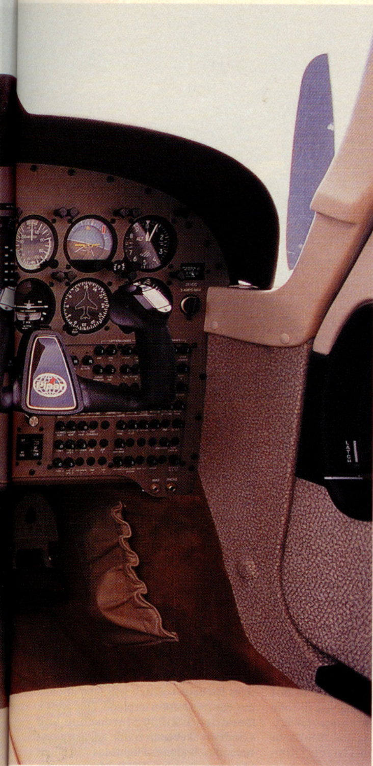
The Seneca V panel, with its vertical engine gauges and digital displays, looks like it would be right at home in a twin turboprop. Optional copilot instruments add $8,305 to the price tag, but leather seats are standard equipment.
